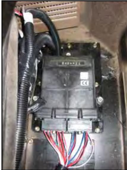
1. Insert the two large, rectangular connectors of the node harness (P/N 115-4001-157) into the correct ports of the node, tightening the bolts on the harness connectors to secure the connections.
