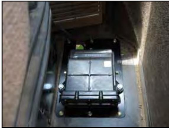
1. Install the SmarTrax MD node on the node mounting bracket (P/N 107-0172-084) using three 3/8"-16 zinc flanged lock nuts (P/N 312-1001-164).
