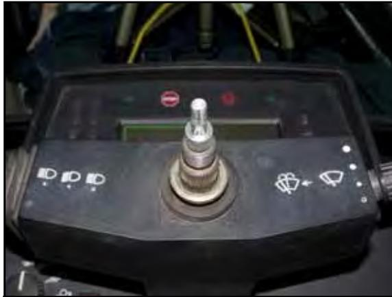
5. Using the steering wheel puller, remove the steering wheel from the steering column.
