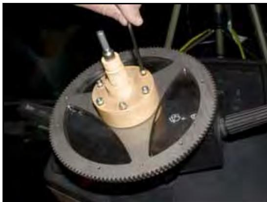
8. Install and tighten the spline assembly bolts to secure the male spline adapter to the ring gear and female spline adapters.
