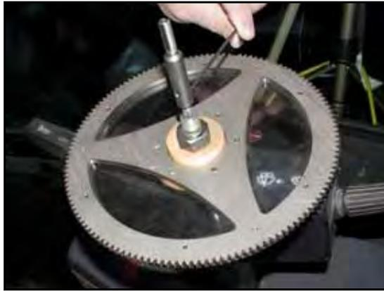
5. Tighten the set screws in the telescope adapter assembly.
