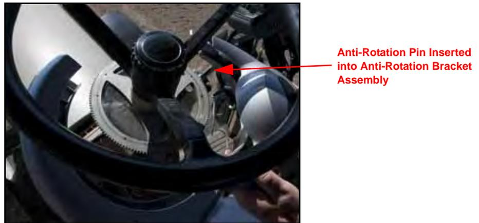
3. Insert the anti-rotation pin into the installed flanged bearing (P/N 325-0000-036) on the anti-rotation bracket assembly.
