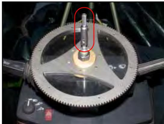
4. Install the telescope adapter assembly (P/N 063-4001-017) on the machine's telescope rod aligning the set screws with the flat part of the stem.
