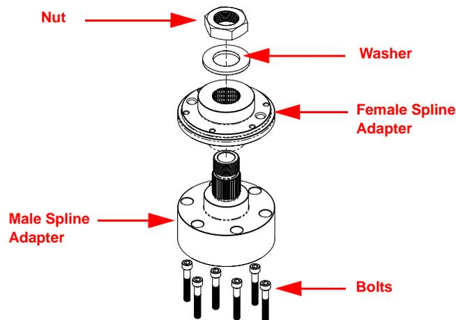
1. Locate the 7/8" 36 tooth spline adapter assembly (P/N 063-4001-015).
