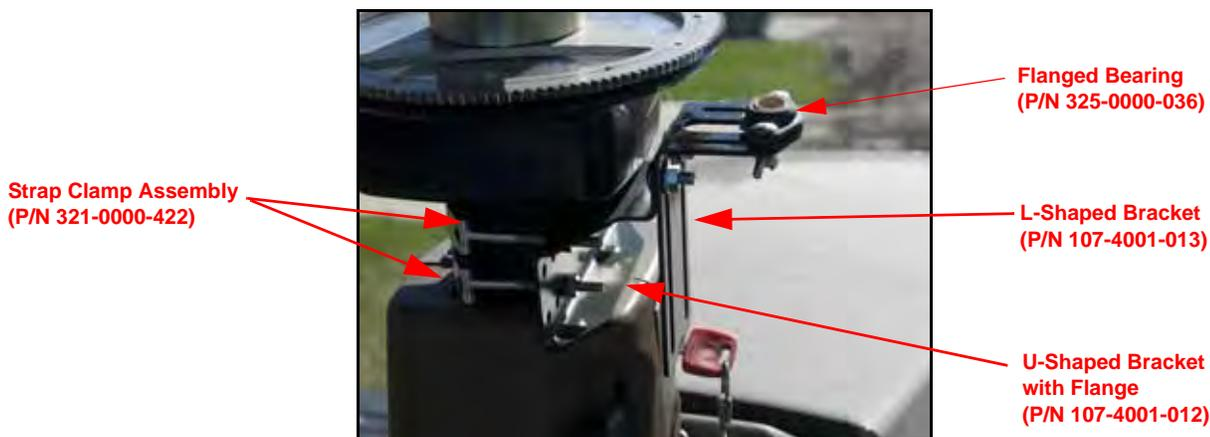
5. Secure the L-shaped bracket to the installed U-shaped bracket using two 5/16"-18 x 3/4" carriage bolts (P/N 311-0069-111) and two 5/16"-18 zinc flanged lock nuts (P/N 312-1001-184).
