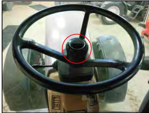
1. Remove the cap from the center of the steering wheel.
