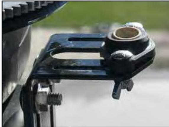
4. Install the 1/2" plastic flanged bearing (P/N 325-0000-036) on the short leg of the L-shaped bracket (P/N 107-4000-013) using two #10-24 wing nuts (P/N 312-3000-013).
