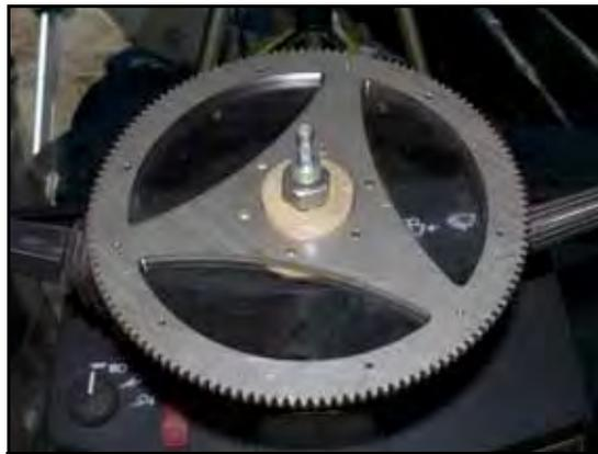
3. Place the ring gear assembly over the female spline adapter with the black ring facing down and the holes in the ring gear aligned with the holes in the female spline adapter.
