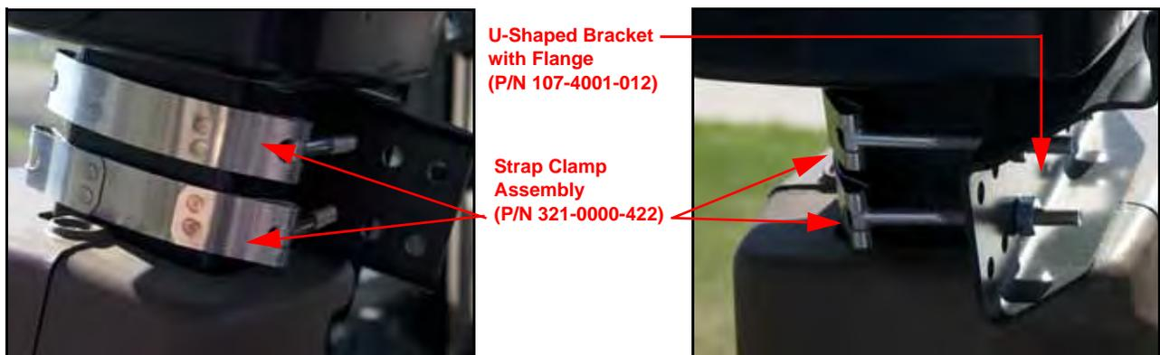
2. Secure the U-shaped bracket (P/N 107-4000-012) to the steering column using the two 4" strap clamp assemblies (P/N 321-0000-422) and supplied nuts.
