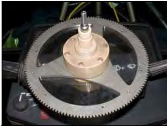
6. Align the bolts holes in the male spline assembly with the holes in the ring gear assembly.
