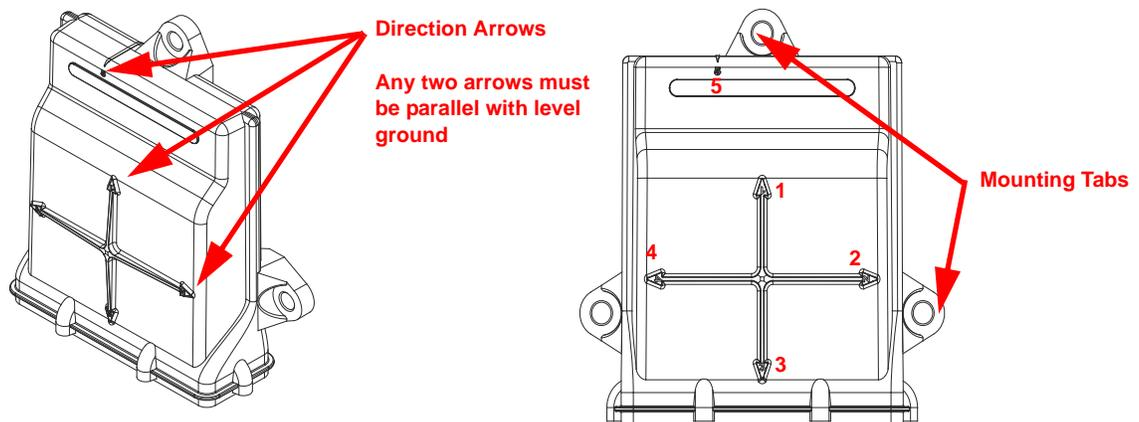
Identify the node mounting location appropriate for the machine's cab configuration. When choosing the location for the SmarTrax MD node, consider the following points:
