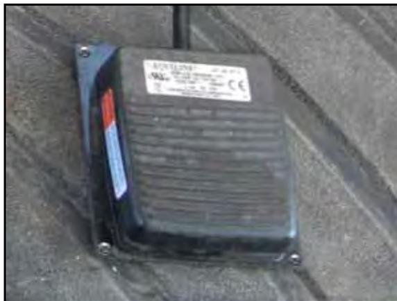
1. Select a suitable location for the foot switch (P/N 063-0173-593) to be installed.
