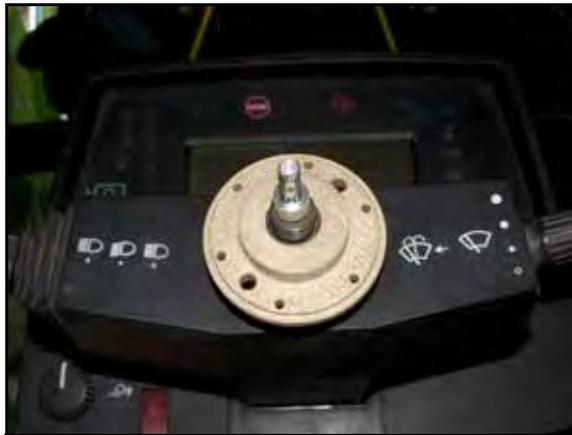
1. Install the female spline on the machine's steering column.
