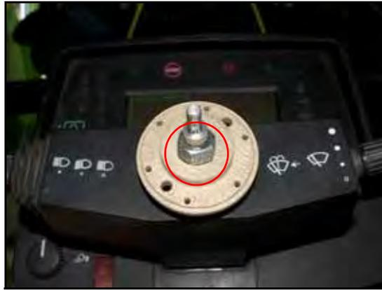
2. Install the machine's steering wheel nut that was removed in step 4 of the *Remove the Steering Wheel* section on page 7 over the installed telescope and female spline adapter.
