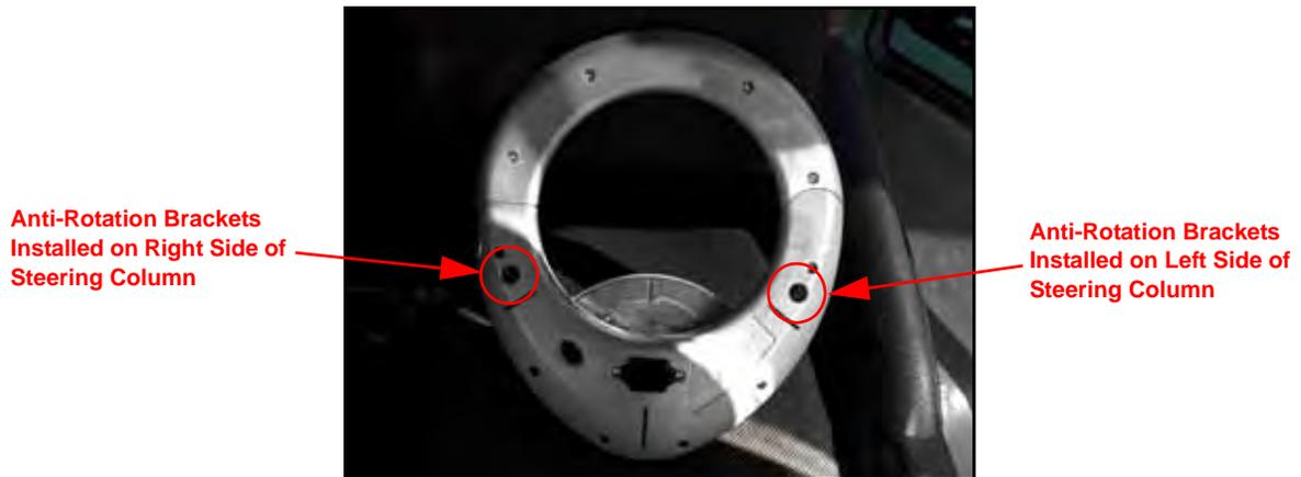
1. Determine the anti-rotation pin (P/N 107-4001-004) installation location on the mechanical drive (P/N 063-4001-010) based on the anti-rotation bracket installation location.
