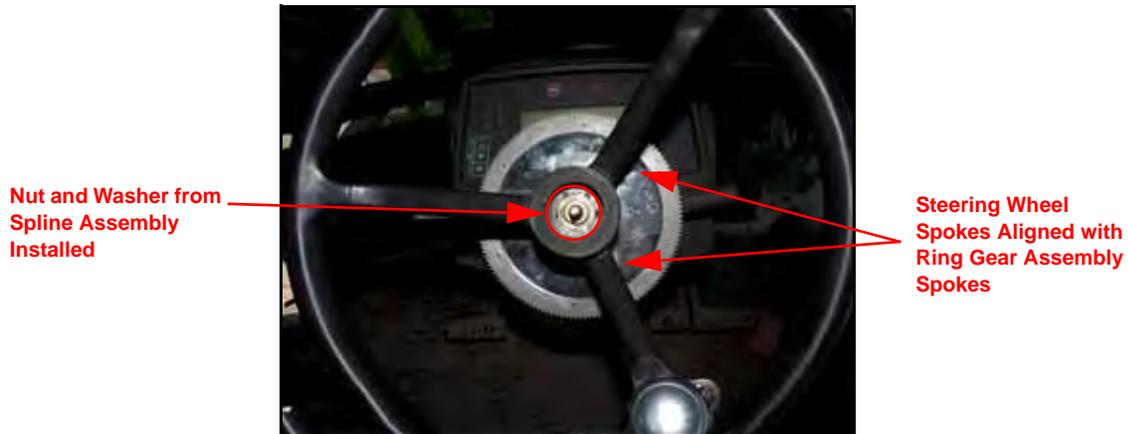
1. Align the spokes of the machine's steering wheel with the spokes on the installed ring gear assembly.
