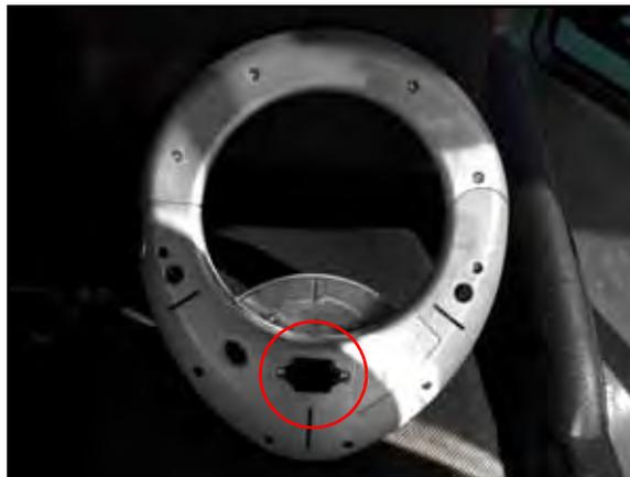
4. Connect the 8-pin Deutsch connector from the node harness into the 8-pin port of the mechanical drive (P/N 063-4001-010).
