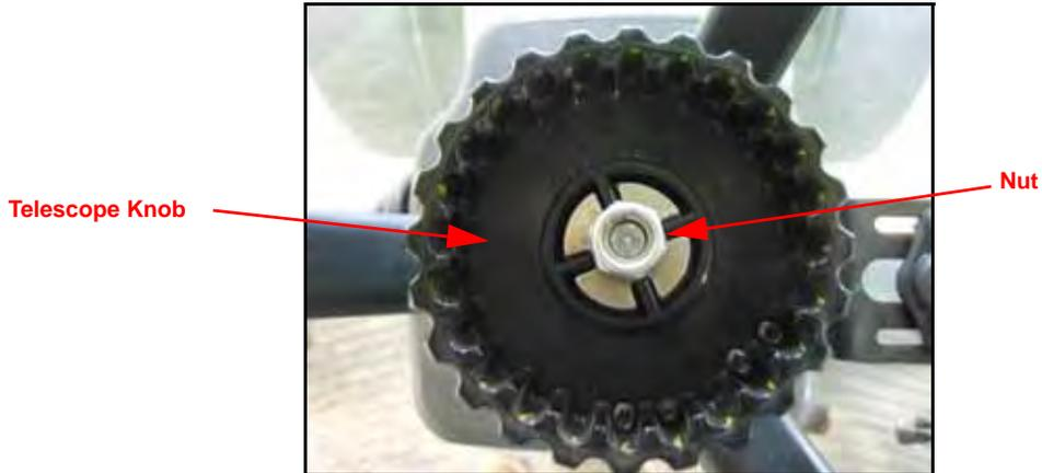
2. Remove the nut used to secure the telescope knob.
